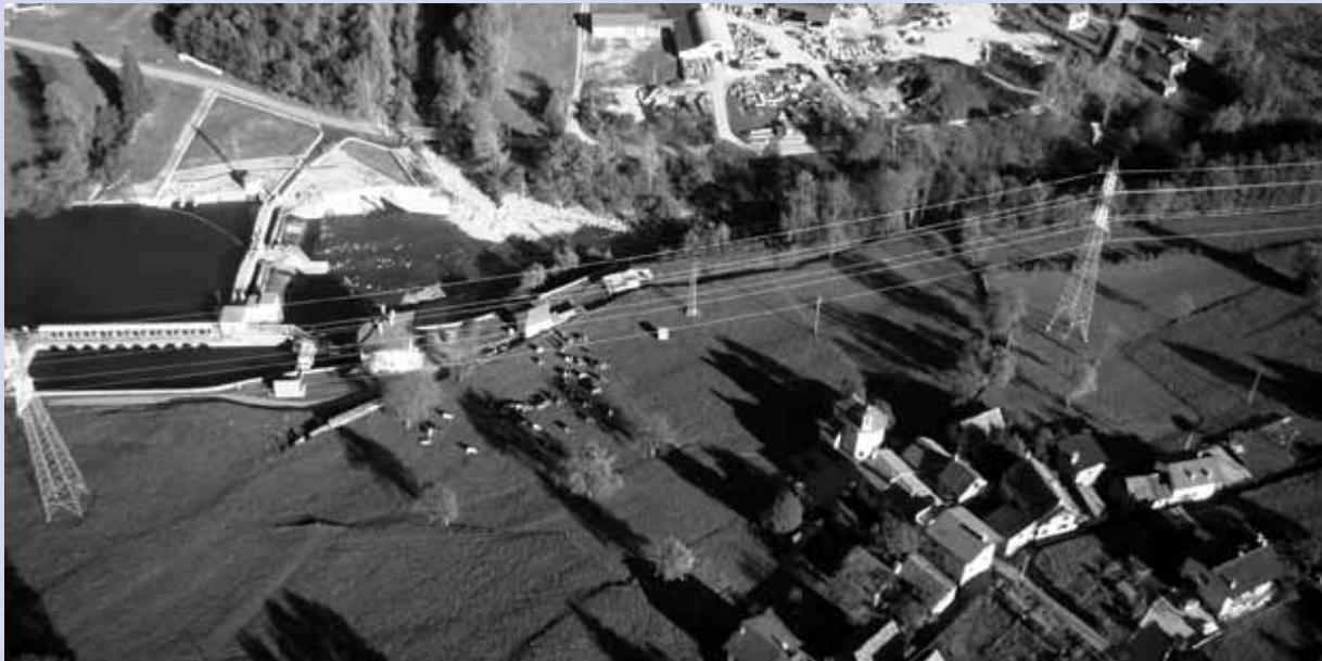
In the second half of 2009, Terna started the LIDAR (Laser Imaging Detection and Ranging) project, with the objective of creating a geo-referred platform of the National Transmission Grid thanks to the use of laser imaging by helicopter.
